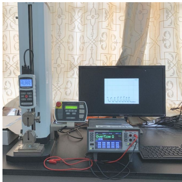
Figure S2. Photograph of the experimental testing platform composed of a digital multimeter and a universal testing machine.
