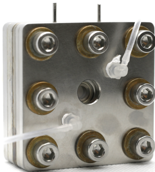
Figure S1. Optical images of the bicarbonate flow cell for operando Raman measurements
