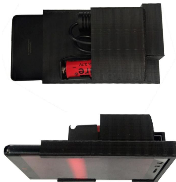
Figure S23. Actual device design of smartphone fluorometric sensing platform.
