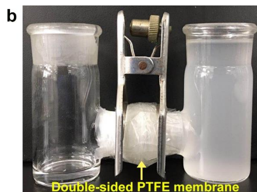
Figure S7. Separation of NE1 by commercial (a) double-sided PVDF membrane and (b) double-sided PTFE membrane under gravity in the H-shape separation apparatus.
