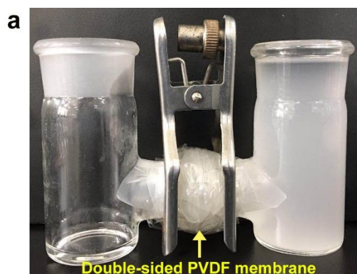
Figure S7. Separation of NE1 by commercial (a) double-sided PVDF membrane and (b) double-sided PTFE membrane under gravity in the H-shape separation apparatus.
