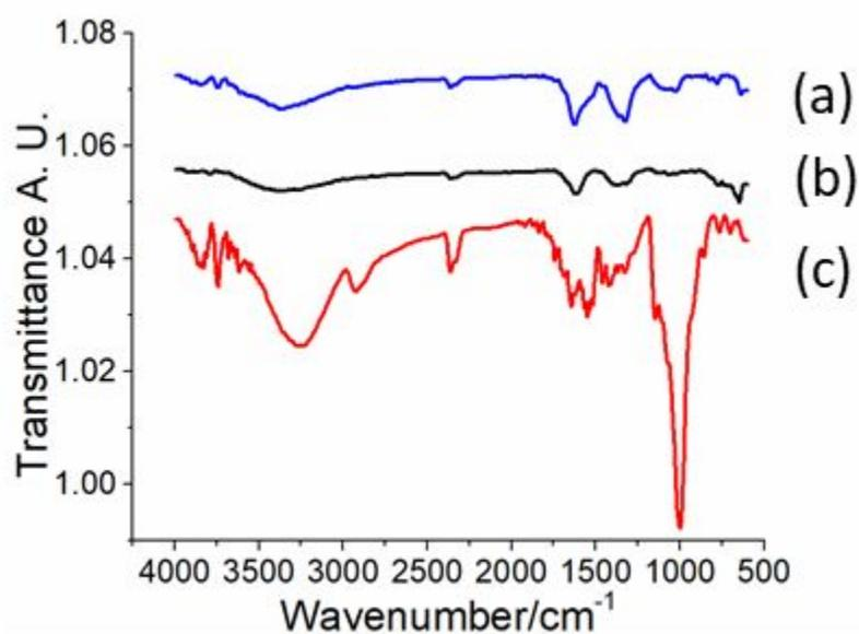
**Figure S1.** FTIR Spectra of (a) Alginate-AA-LDHs and glycerol coating solution (b)
