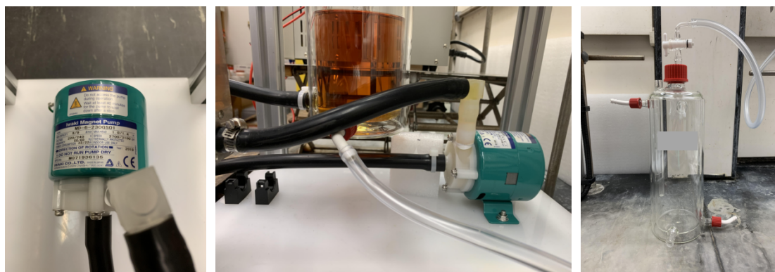
Figure S5. (Left) Circulating Pump (Center) Pump in a running reaction (Right) 1.0 L jacketed reservoir
