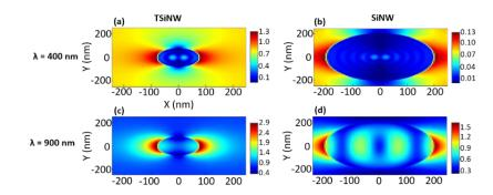
**Figure S1**: Electric field enhancement around conventional SiNWs (b and d) and TSiNWs (a and c) at 400 and 900 nm, respectively.
