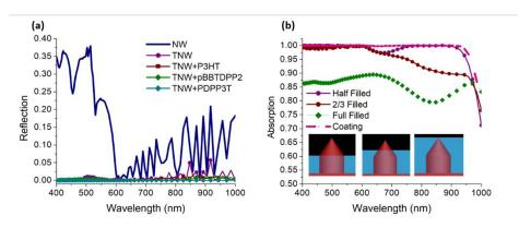
**Figure S2:** (a) Comparison between the reflection of conventional SiNWs, TSiNWs and TSiNWs coated with different polymers. (b) Absorption simulated for different configurations for the polymer with TSiNWs.
