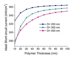
**Figure S5:** Ideal short circuit current calculated for different polymer coating thickness at different TSiNW diameters.
