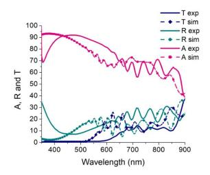
Figure S4: simulated (sim) and measured (exp) absorption of 1.2  $\mu$ m flat a-Si layer and 200 nm PDPP3T on top.
