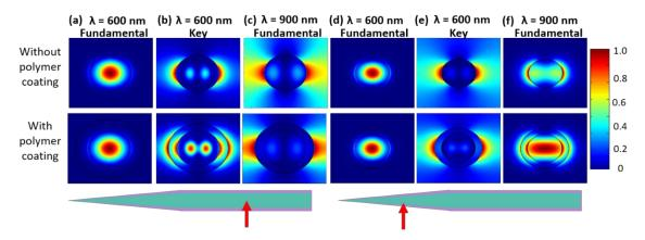
**Figure S6:** (a,c) The fundamental mode and (b) the key mode with and without polymer coating at multiple wavelengths in the location indicated by the red arrow in the TSiNW underneath. (d,f) The fundamental mode and (e) the key mode in the tapered part of the NW as indicated by the red arrow in the TSiNW underneath.
