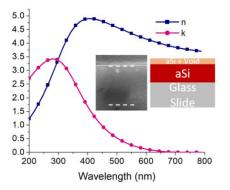
**Figure S3:** Optical constants of the deposited aSi thin film as determined by the ellipsometry. The inset is the model built in the ellipsometry software.
