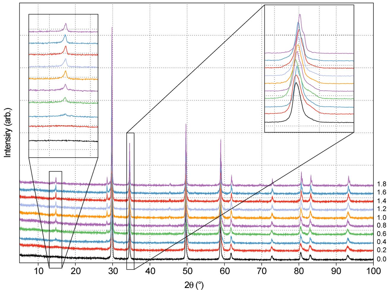
Figure S1.1. Powder XRD patterns for  $Y_2Hf_{2-x}Sn_xO_7$ .
