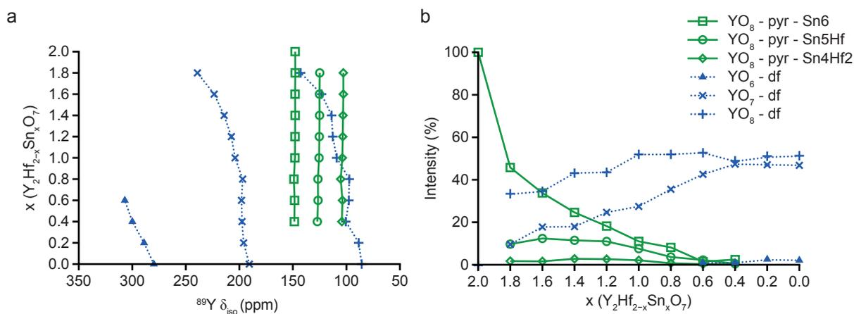
**Figure S4.2.** Plot showing the variation of (a) chemical shifts and (b) integrated intensities of resonances in the  $^{89}\text{Y}$  MAS NMR spectra of  $\text{Y}_2\text{Hf}_{2-x}\text{Sn}_x\text{O}_7$  with nominal composition. Resonances attributed to the pyrochlore and defect fluorite phases are denoted pyr and df, respectively. For the pyrochlore phase, the B site NNN arrangement for each environment is also shown.
