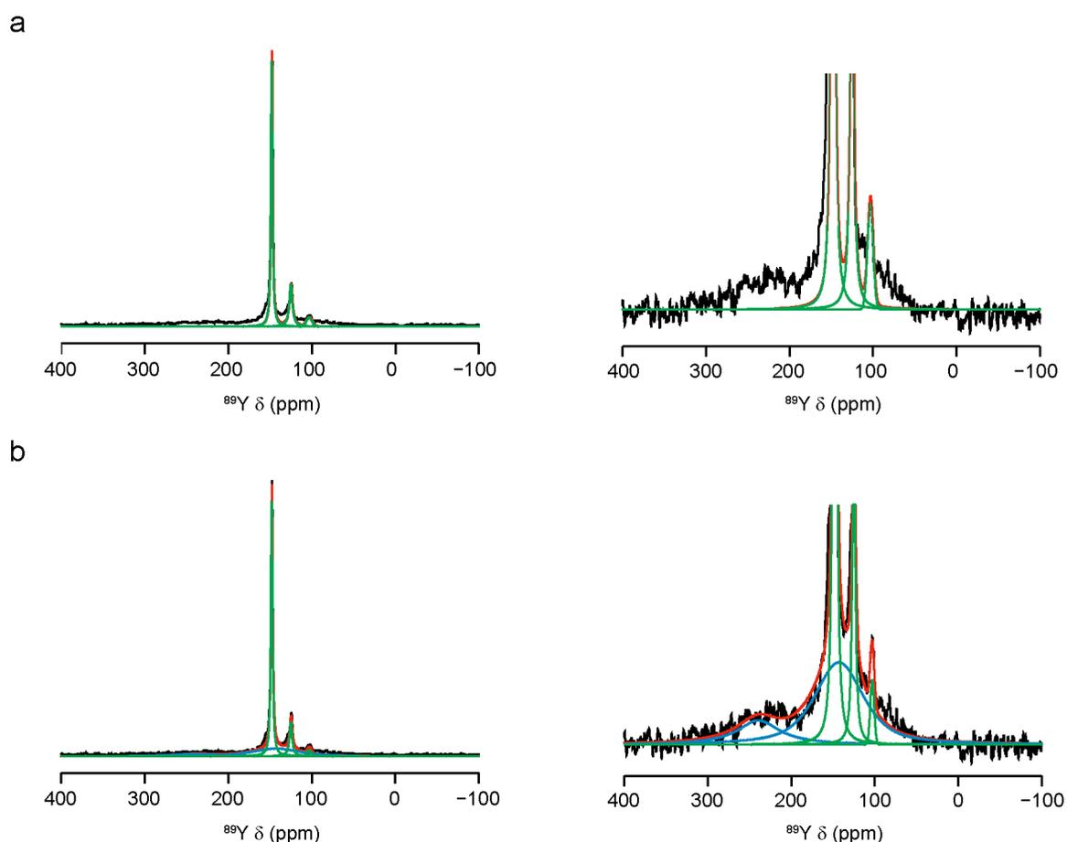
**Figure S4.1.** Analytical fits and corresponding (vertical) expansions of the  $^{89}\text{Y}$  MAS NMR spectrum of  $\text{Y}_2\text{Hf}_{0.2}\text{Sn}_{1.8}\text{O}_7$ . In (a), the spectrum is fitted without the inclusion of the broad resonances associated with the disordered defect fluorite phase. In (b), two broad resonances are included. The green, blue and red lines denote the analytical fit for the pyrochlore phase, defect fluorite phase and all resonances, respectively.
