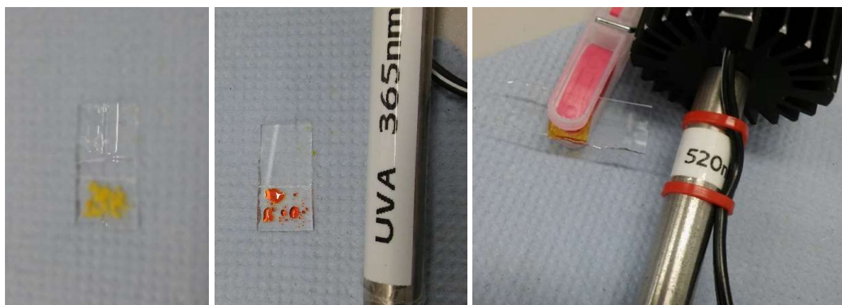
Figure S6 | Photographs of the different steps in the cohesion methodology. The applied methodology for conjoining glass slides with AIZ adhesives. (Left) Weighing out 2.1 mg of arylazo-3,5-dimethylisoxazole within a 1.4 x 1.0 cm surface of a glass slide. (Middle) Irradiation at 365 nm to cause a solid-to-liquid phase transition. (Right) pressing two 1.4 x 1.0 cm overlapping glass surfaces together and irradiating at 520 nm to induce the liquid-to-solid phase transition.
