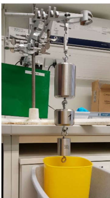
Figure S13 | Maximum weight bearing at plexiglass (PMMA) slides cohered with AIZ 2. Suspension of plexiglass (PMMA) slides conjoined with 2.2 mg of compound 2 at a 1.0 by 1.4 cm overlapping surface area, capable of bearing a load of up to 3.5 kg without rupture.
