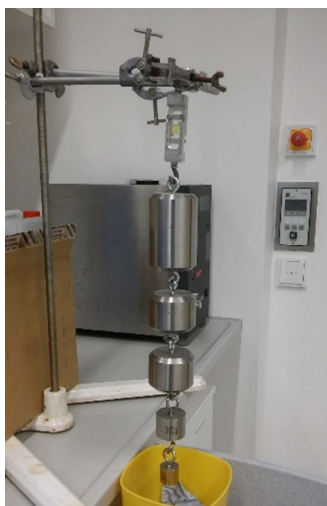
Figure S9 | Maximum weight bearing at glass slides cohered with AIZ 2. Suspension of glass slides conjoined with 2.1 mg of compound 2 at a 1.0 by 1.4 cm overlapping surface area, bearing a load of 4.4 kg without breaking.
