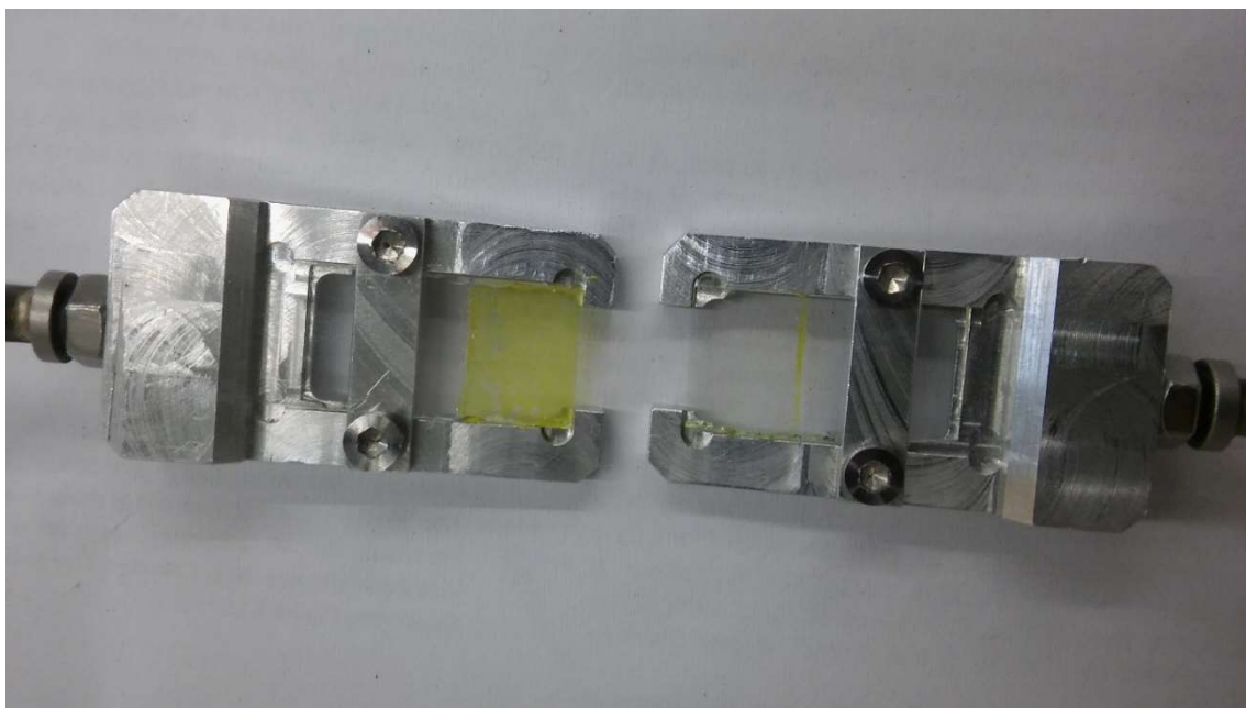
Figure S7 | Photograph of formerly cohered slides after UV-induced adhesive failure. The glass slides after photochemically induced separation of compound 1 from the interface at the right-hand glass slide.
