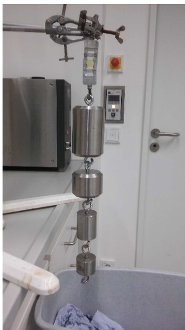
Figure S12 | Maximum weight bearing at conjoined plexiglass (PMMA) and glass with AIZ 2. Suspension of glass slides conjoined with 2.1 mg of compound 2 at a 1.0 by 1.4 cm overlapping surface area, bearing a load of 3.8 kg without rupture.
