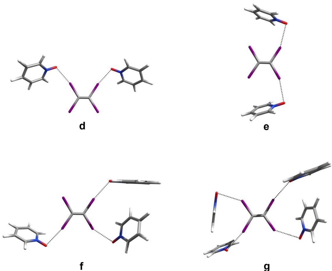
**Figure S9.** Different XB motifs of **1** and  $\text{C}_2\text{I}_4$  optimized at PBE0-D3/def2-TZVP level of theory.
