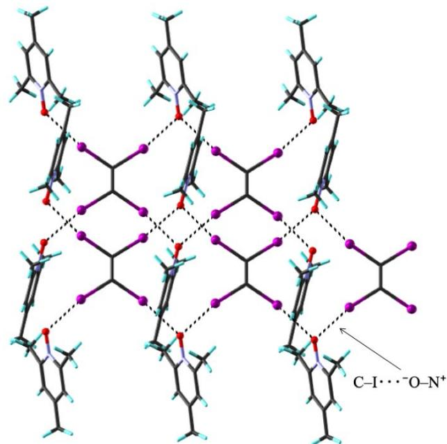
**Figure S2.** X-ray crystal structure packing of  $7 \cdot \text{C}_2\text{I}_4$ . The black-dotted lines are  $\text{C}-\text{I}\cdots\text{O}-\text{N}^+$  XBs.
