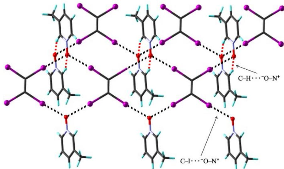
**Figure S1.** X-ray crystal structure packing of  $3 \cdot \text{C}_2\text{I}_4$ . The black-dotted lines are  $\text{C}-\text{I}\cdots\text{O}-\text{N}^+$  XBs and red-dotted lines represent  $\text{C}-\text{H}\cdots\text{O}-\text{N}^+$  interactions.
