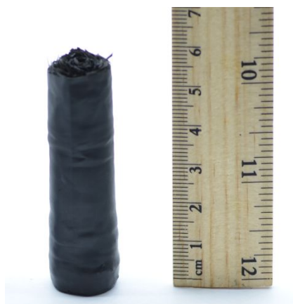
Figure S2. A large FAT electrode with diameter of 18 mm and height of ~55 mm for potential 18650 cylindrical cell application.
