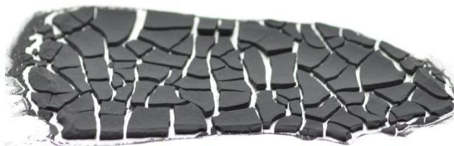
Figure S3. Photo image of slurry-cased electrode. After drying, cracks occurred in the thick electrode.
