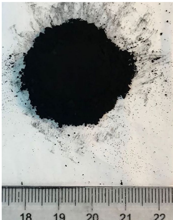
Figure S1. Massive production of SA-Ag/NC. By our synthesis method with 0.2 g carbon black, 0.109 g silver nitrate and 2 g urea, one batch of produced SA-Ag/NC has a volume of 4 mL and the mass of 460 mg, which are limited only by the capacity of the porcelain boat used in the pyrolysis. If larger porcelain boats are used, the production yield of SA-Ag/NC can be easily scaled up.
