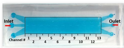
Figure S1. Photograph of microfluidic chip used in this manuscript. Blue pigment was injected to light the channel.
