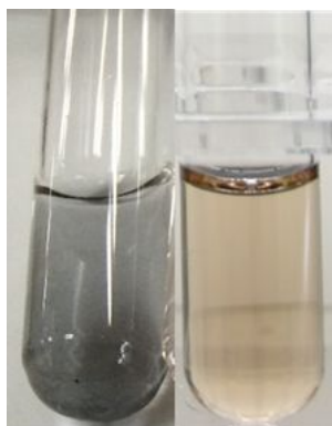
Figure S2. AuNPs prepared by normal mixing in beaker (left) and MIVM (right). All the chemicals were at same concentrations.
