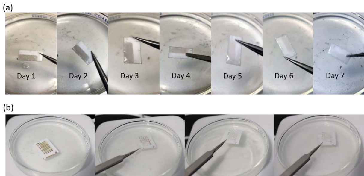
Figure S3. Progressive dissolutions of 2D MoS 2 layers integrated on; (a) a paper substrate, and (b) a paper substrate with Au electrode contacts.
