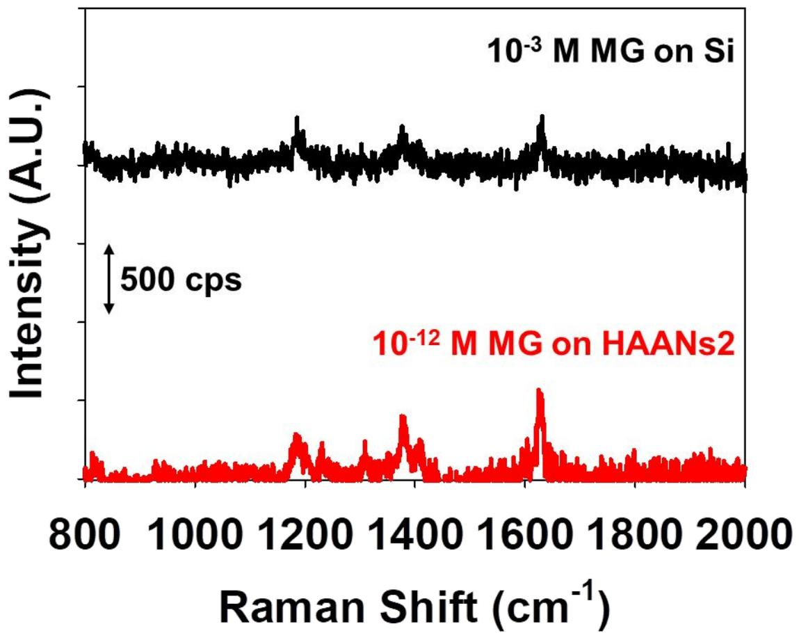
**Figure S13.** Representative Raman spectra of 10<sup>-3</sup> M MG on bare Si wafer and 10<sup>-12</sup> M MG on HAANs2
