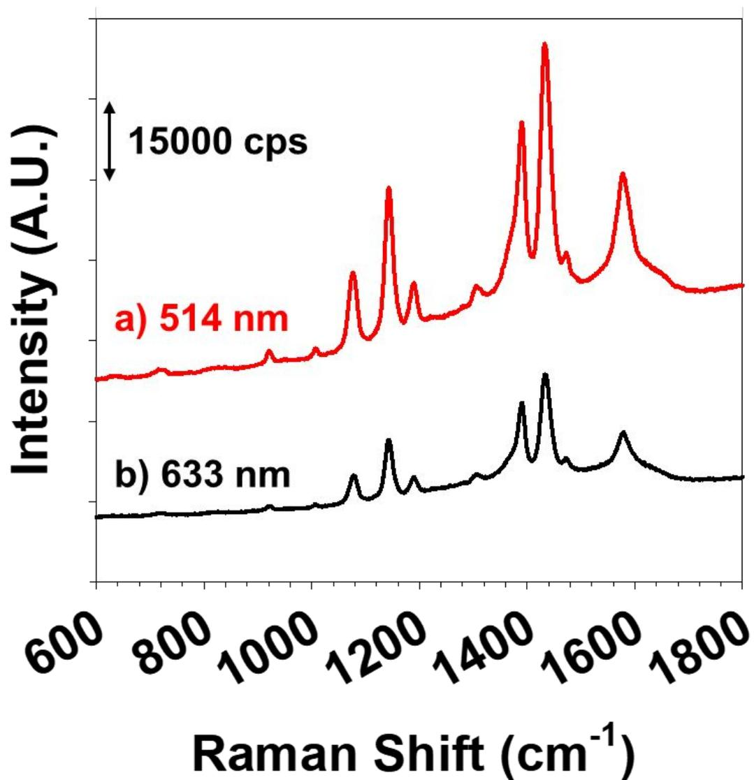
**Figure S12.** Representative Raman Spectra of  $1 \times 10^{-5}$  M p-ATP treated HAANs2 under the irradiation of a) 514 nm and b) 633 nm laser.
