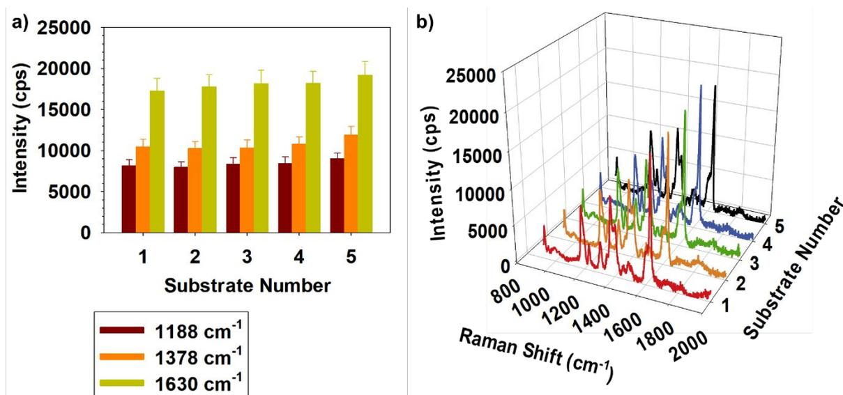
**Figure S10.** Synthetic reproducibility of HAANs2. The peak intensities of  $10^{-5}$  M MG were measured from different 5 substrates from different SDAs, under 514 nm laser irradiation.
