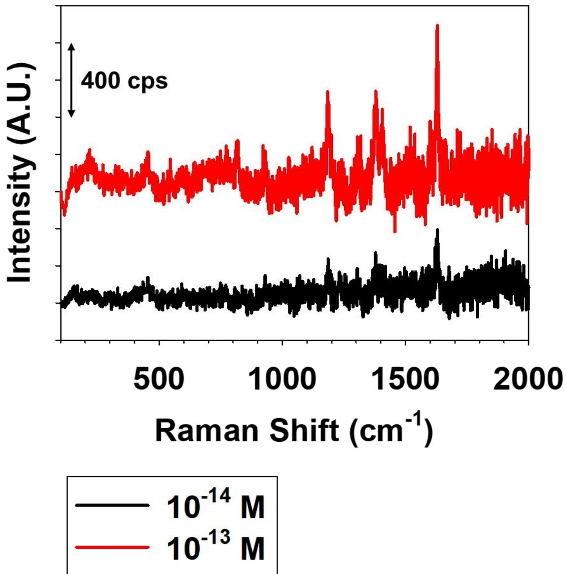
**Figure S14.** SERS spectra of  $1 \times 10^{-14}$  M and  $1 \times 10^{-13}$  M of MG treated HAANs2 in **Figure 6a**.
