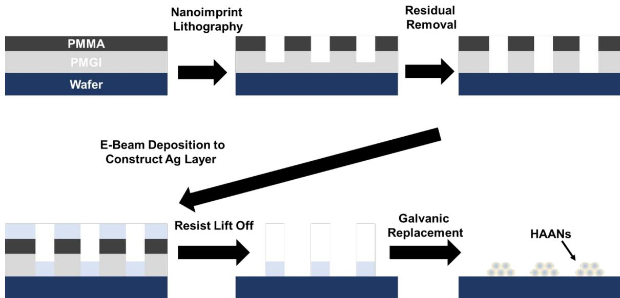
**Figure S1.** Schematic illustration of overall process in this research: Nanoimprint lithography (NIL) was performed and resist residual was removed by consecutive dry etching and wet chemical dissolution of PMGI (polymethylglutarimid) E-Beam deposition was conducted to construct Au layer. Lift-off process to erase resist with AZ-MIF 300 developer was performed to generate SDAs. Thereafter, H<sub>Au</sub>Cl<sub>4</sub> aqueous solution was injected to HAANs via galvanic replacement.
