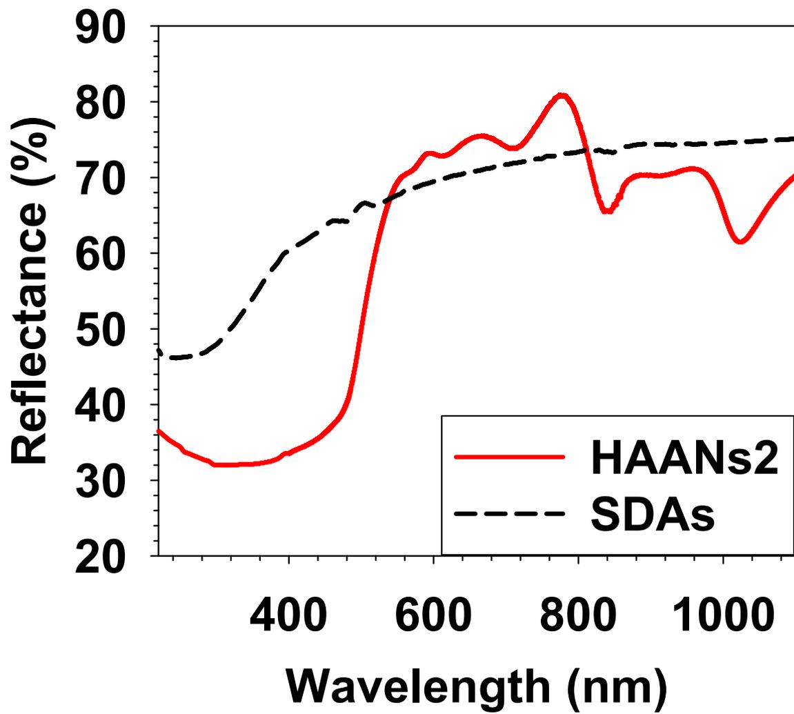
**Figure S11.** The reflectance spectrum of SDAs (black dashed line) and HAANs2 (red line).
