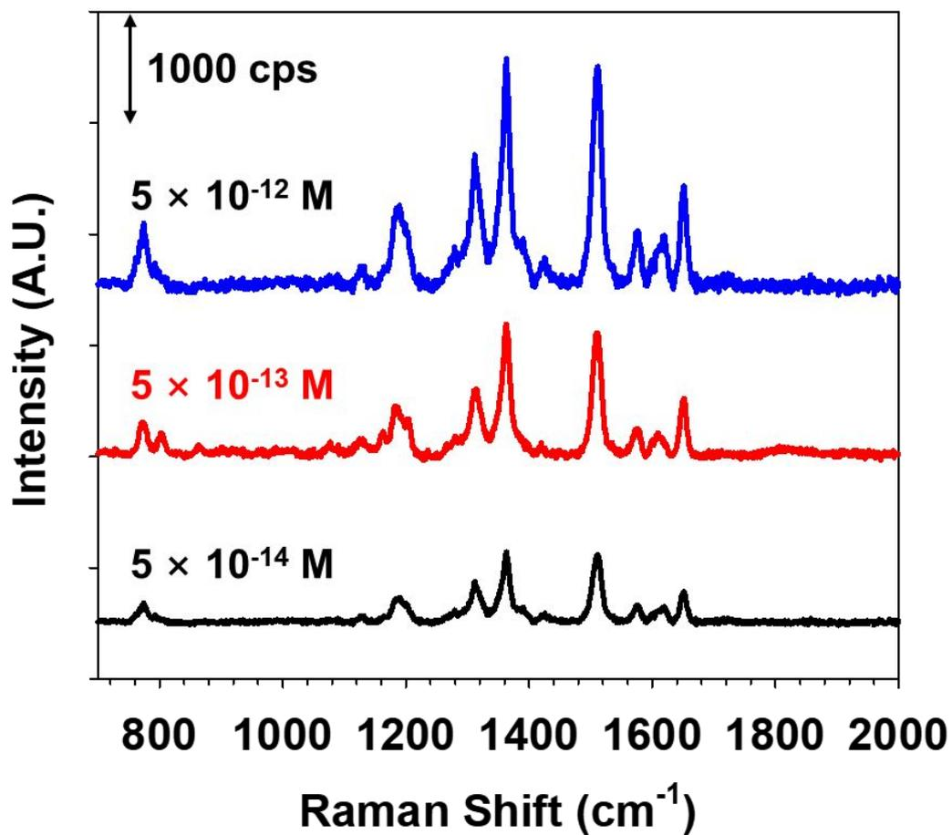
**Figure S15.** Different SERS spectra of HAANs2 with respect to the different rhodamine 6G concentrations ( $5 \times 10^{-14}$  M to  $5 \times 10^{-12}$  M) to determine limit of detection (LOD) under 514 nm irradiation.
