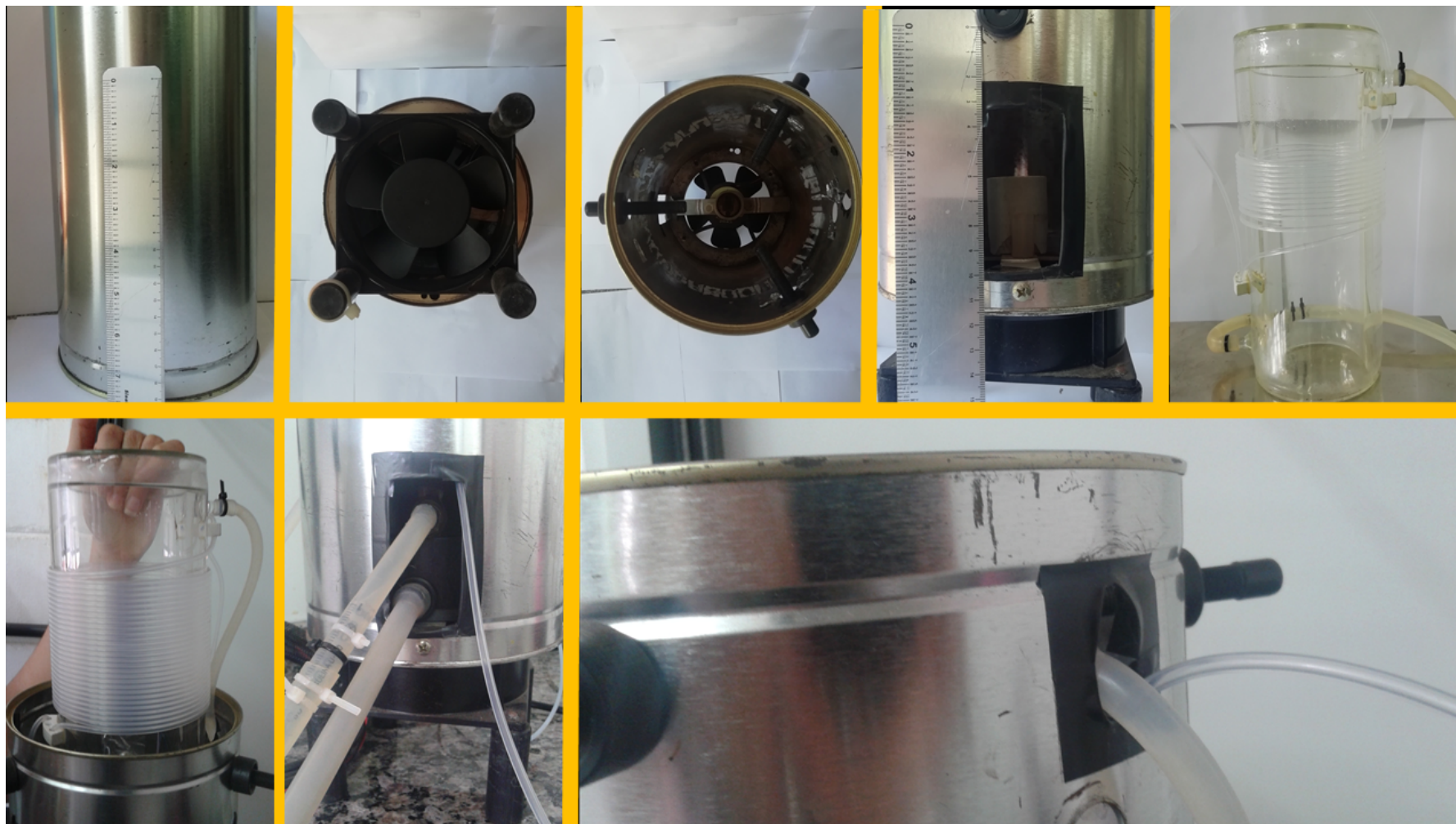
Figure S5. Construction of the photochemical reactor for continuous flow reaction at low temperature
