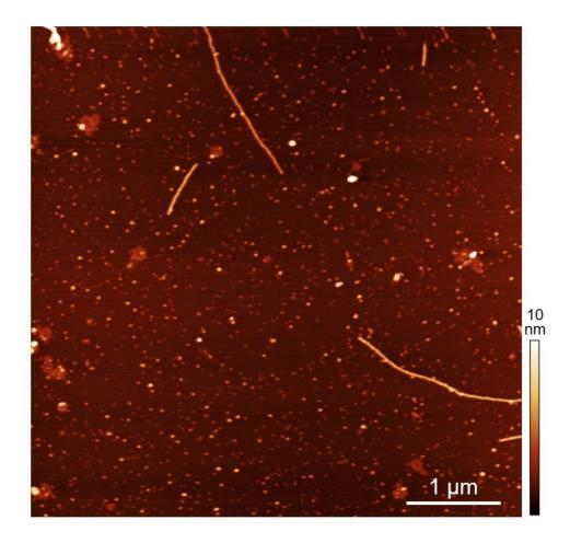
Figure S2. AFM height image of A $\beta$ 40 amyloid fibrils formed on mica by incubation at 37 °C for 24 hours. The concentration of A $\beta$ 40 in PBS solution is 1  $\mu$ M.
