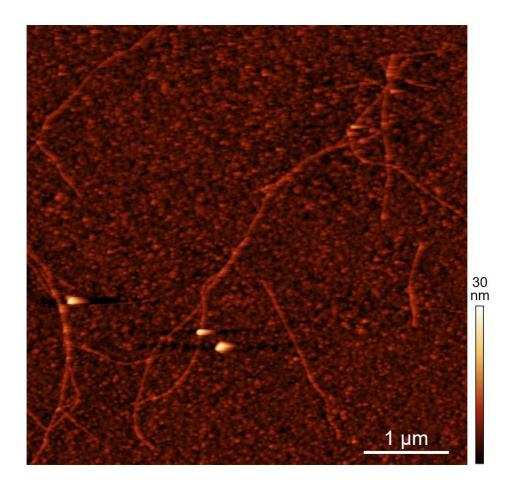
**Figure S1**. AFM height image of A $\beta$ 40 amyloid fibrils formed on plasma treated polystyrene surface by incubation at 37 °C for 24 hours. The concentration of A $\beta$ 40 in PBS solution is 1  $\mu$ M.
