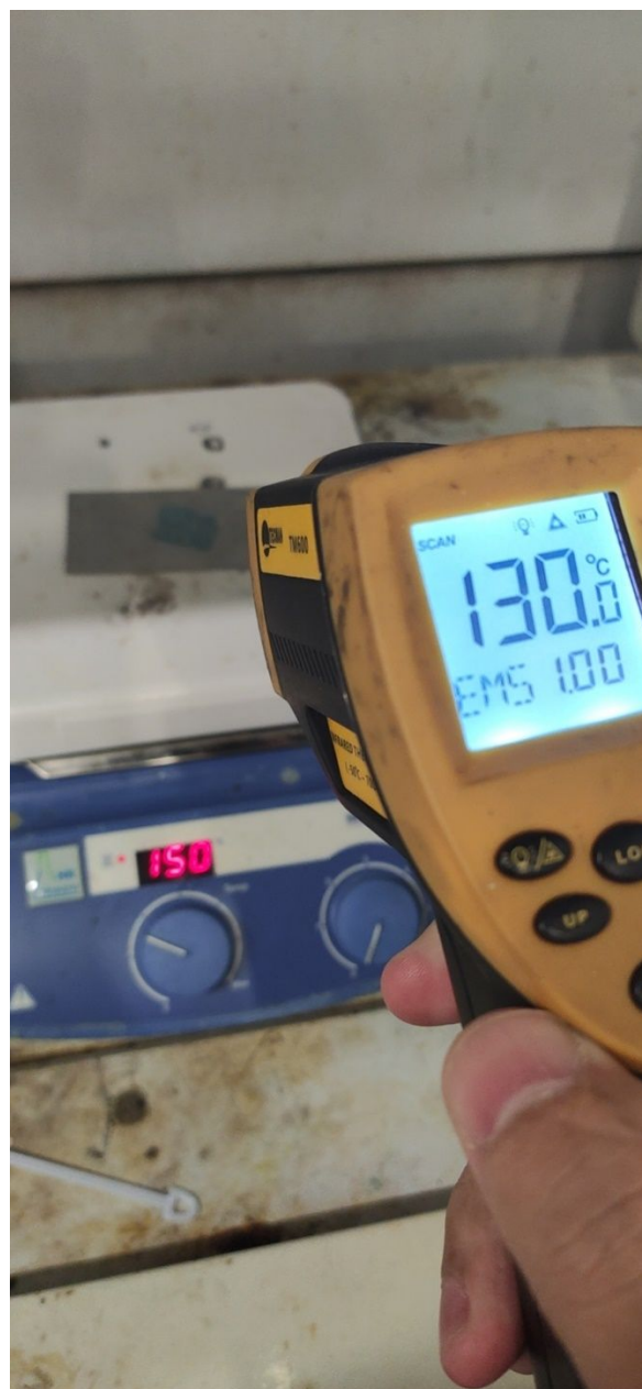
Figure S3. The experimental setup for measuring the melting point of the pristine mask. The hotplate was set to 150 °C, and the surface temperature of the pristine mask was measured to be 130 °C.
