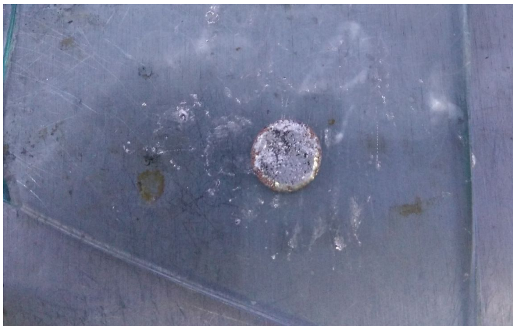
Figure S7. Successful preparation of the Na-K@Cu foam membrane electrode using the transferring chamber of the glovebox as the special chamber of the vacuum infiltration method.
