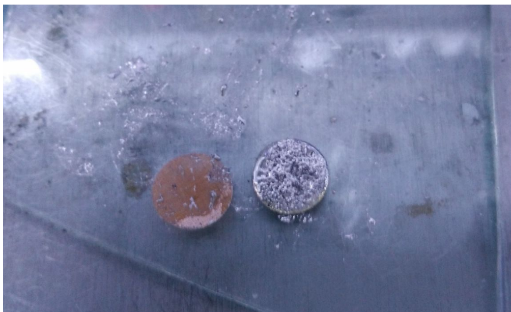
Figure S8. Unsuccessful preparation of the Na-K@Cu mesh. The experiment was conducted utilizing the same experiment design in Figure S4 with Cu foam and Cu mesh both beneath the Na-K alloy.
