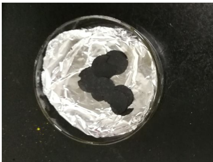
Figure S11. The free-standing \text{Na}_3\text{V}_2(\text{PO}_4)_3 electrode used for the Na-K-Sn@mesh- \text{Na}_3\text{V}_2(\text{PO}_4)_3 full cell with high areal loading of \text{Na}_3\text{V}_2(\text{PO}_4)_3 active material.
