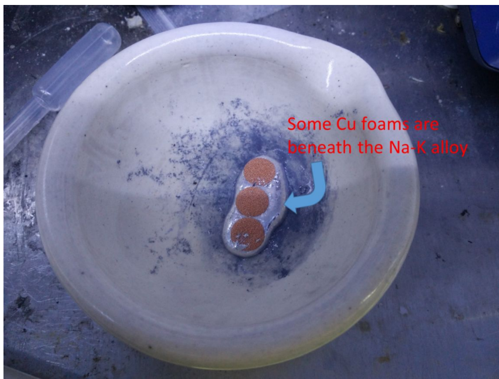
Figure S6. Experiment image of using vacuum infiltration method to reproduce Na-K@Cu foam.
