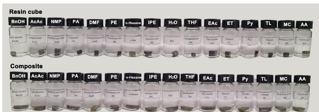
Figure S2. Samples soaked in different solvents (0 day)
