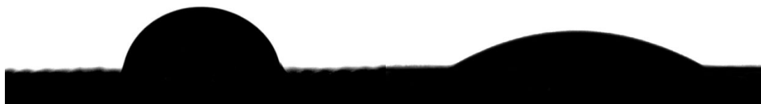
Figure S3. The initial contact angles for the hydrophilic side of a) Janus cotton fabric and b) corresponding Janus composite fabric. Oxidation time: 2 h.
