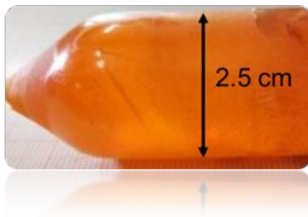
Figure S1. Photograph of the fabricated CsPbBr 3 perovskite crystals or ingot.
