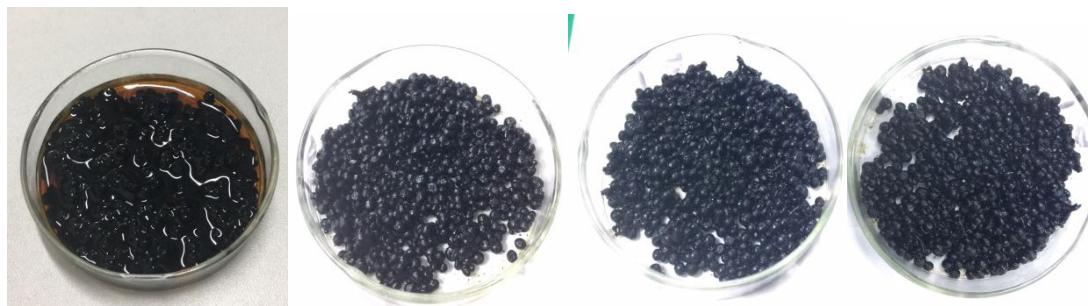
Figure S15. optical image of multi layer samples : a. immersed in adsorbed water ( one night at ambient condition), b. 5 cycles, c. ten cycles. and d. 20 cycles.
