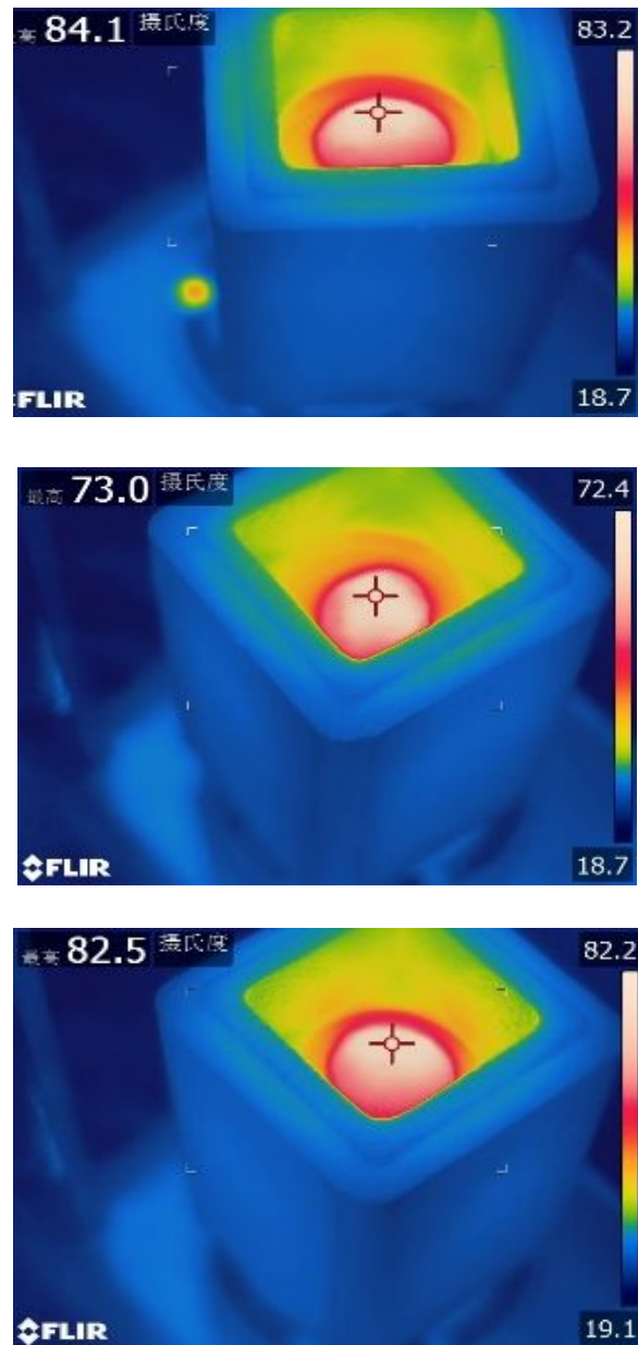
Figure S8. The surface temperature of C/FCNT (top), L/FCNT (middle) and Bina/FCNT(bottom) under one sun irradiation.
