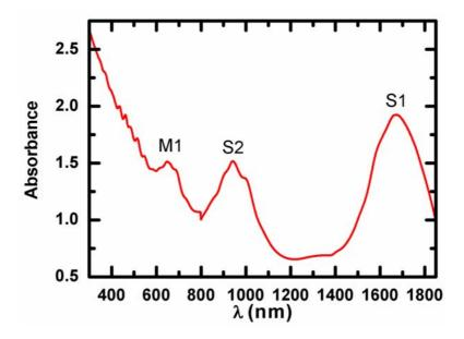
Supplementary Figure 1. Optical absorption spectrum of length separated SWNTs dispersed in  $D_2O$  with 1 weight % sodium cholate. The SWNT concentration is  $\sim 100 \ \mu g/ml$ .
