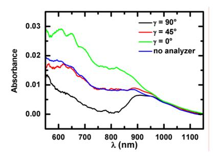
**Supplementary Figure 5.** Polarization dependent absorption spectra of length separated SWNTs in 1 w % SDBS, deposited with  $\nu$ = 80 MHz and  $V_{pp}$  = 80 V. Raw data was smoothed and offset for better comparison.
