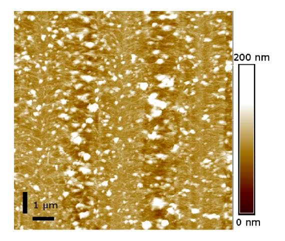
**Supplementary Figure 2.** Atomic force microscope image of a typical sample of nanotubes deposited onto an array of interdigitated electrodes. The areas with light brown background correspond to three electrodes, the darker background marks the gaps. The thickness of the nanotube film was determined to  $\sim 60$  nm.
