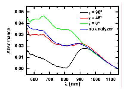
**Supplementary Figure 6.** Polarization dependent absorption spectra of centrifuged SWNTs in 1 w % SDBS, deposited with  $\nu$ = 80 MHz and  $V_{pp}$  = 80 V. Raw data was smoothed and offset for better comparison.
