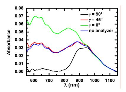
**Supplementary Figure 3.** Polarization dependent absorption spectra of length separated SWNTs in 1 w % SDBS, deposited with v = 10 MHz and  $V_{pp} = 40$  V. The raw data was smoothed and a linear background was subtracted. Metallic and small diameter semiconducting nanotubes are well aligned parallel to the electric field, while semiconducting nanotubes are randomly oriented.
