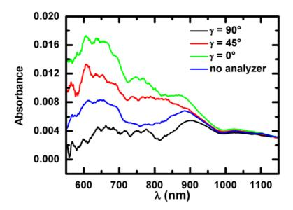
**Supplementary Figure 4.** Polarization dependent absorption spectra of length separated SWNTs in 1 w % SDBS, deposited with  $\nu$ = 80 MHz and  $V_{pp}$  = 40 V. The raw data was smoothed and offset for better comparison. As reported earlier, the amount of deposited nanotubes reduces significantly at high frequencies, resulting in a very low signal intensity and a relatively big measurement error.
