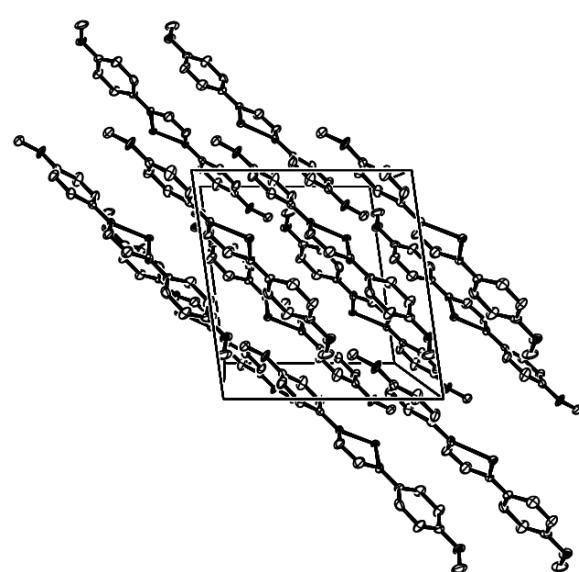
**Figure S4.** Packing diagram for  $(C_5Me_5)_2Yb(dad(H)-p\text{-anisyl})$  (ellipsoids at the 50 % probability level). C<sub>5</sub>Me<sub>5</sub> rings and hydrogen atoms have been omitted for clarity. Shortest inter-molecular contacts between dad-units are ( $C(\text{aromatic})OCH_3 \cdots C(\text{aromatic})$ ) of 3.64 Å and ( $C(\text{aromatic})OMe \cdots C(\text{aromatic})$ ) of 3.55 Å.
