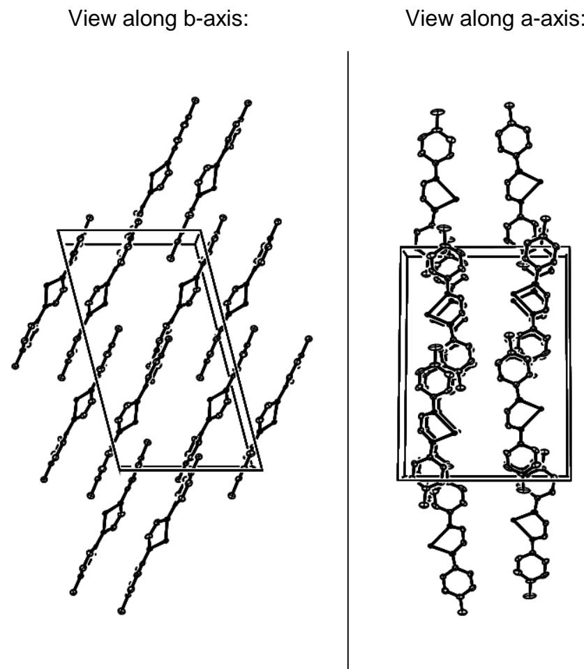
**Figure S3.** Packing diagram for  $(C_5Me_5)_2Yb(dad(H)-p\text{-tolyl})$  (ellipsoids at the 50 % probability level).  $C_5Me_5$  rings and hydrogen atoms have been omitted for clarity. Shortest inter-molecular contact between dad-units ( $C(\text{aromatic})\text{CH}_3 \cdots C(\text{aromatic})$ ) is 3.67 Å.
