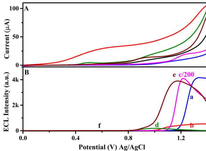
**Figure S2.** (A) LSW and (B) ECL-potential profiles of (a, blue line) GCE|Au NCs/Nafion, (b, red line) GCE|CdSe NCs/Nafion, (c, magenta line) GCE|Ru(bpy)<sub>3</sub><sup>2+</sup>/Nafion, (d, olive line) GCE|CIS/ZnS NCs/Nafion, (e, wine line) GCE|CdTe NCs/Nafion, and (f, black line) GCE|Nafion in 50 mM pH 7.4 Tris-HCl containing 50 mM KNO<sub>3</sub> and 0.1 mM TPrA at 50 mV/s.
