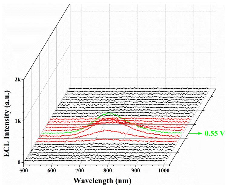
**Figure S4.** Spooling ECL spectra of GCE|CIS/ZnS NCs/Nafion in 50 mM pH 7.4 Tris-HCl containing 50 mM KNO<sub>3</sub> and 50 mM CON<sub>4</sub>H<sub>6</sub> at 50 mV/s. Each spectrum is recorded with 1.0 s time intervals, that is, 50 mV potential intervals during the potential scan.
