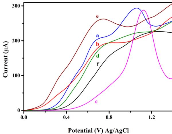
**Figure S1.** DPV profiles of (a, blue line) GCE|Au NCs/Nafion, (b, red line) GCE|CdSe NCs/Nafion, (c, magenta line) GCE|Ru(bpy)<sub>3</sub><sup>2+</sup>/Nafion, (d, olive line) GCE|CIS/ZnS NCs/Nafion, (e, wine line) GCE|CdTe NCs/Nafion, and (f, black line) GCE|Nafion in 50 mM pH 7.4 Tris-HCl containing 50 mM KNO<sub>3</sub> and 50 mM CON<sub>4</sub>H<sub>6</sub>.
