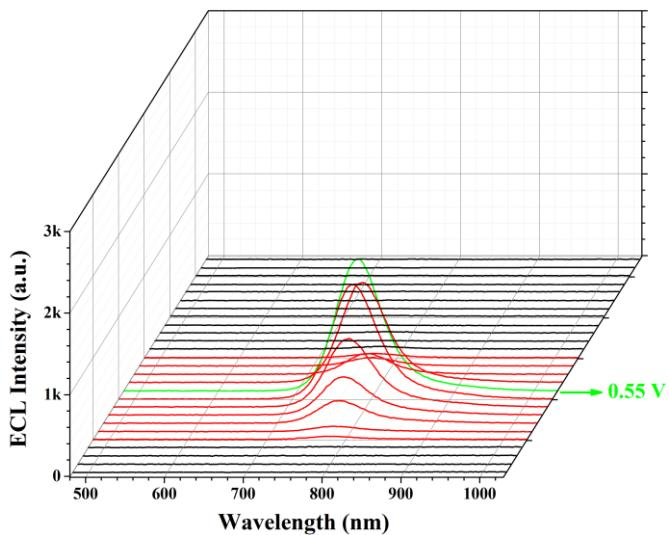
**Figure S5.** Spooling ECL spectra of GCE|CdTe NCs/Nafion in 50 mM pH 7.4 Tris-HCl containing 50 mM KNO<sub>3</sub> and 50 mM CON<sub>4</sub>H<sub>6</sub> at 50 mV/s. Each spectrum is recorded with 1.0 s time intervals, that is, 50 mV potential intervals during the potential scan.
