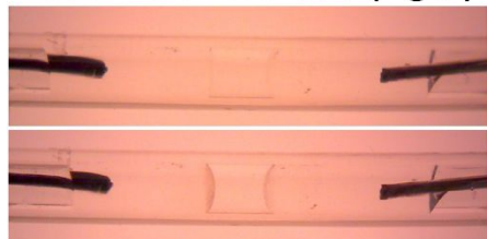
Figure S10. \mu -EME setup. The cathode was located to the left and the anode to the right. For all experiments, the anode was of silver (Ag). The amount of current each system had been exposed to for individual photographs is given next to the photo (mC). The upper photographs show the development of color of phenolphthalein as the pH increases at the cathode with a normal silver electrode. The lower photographs show no pH increase when a sacrificial electrode was used. Voltage: 150 V.
