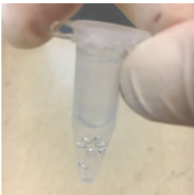
Figure S17. O 2 bubble was produced from the UMOFs@Au NPs solution (10 µg/mL) in the presence of H 2 O 2 (150 µM). The appearance of bubble in the solution showed the highly catalytic activity of UMOFs@Au NPs in the production of O 2 .
