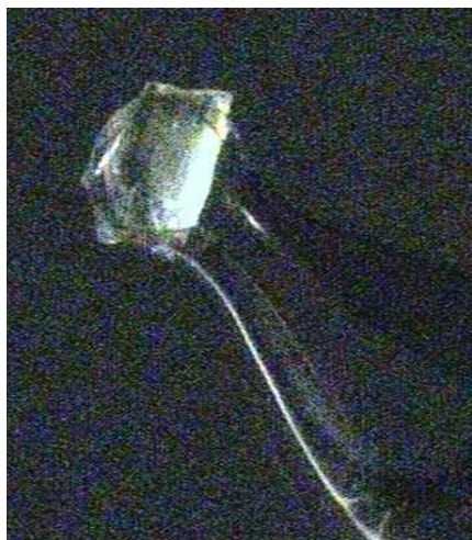
Figure S3: A shock-cooled single-crystal of 7 mounted on a holder in perfluoroether oil.
