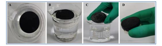
**Fig.S1** (A-B) The PPy-coated VMP foam immersed in water for 4 months. (C-D) Removed PPy-coated VMP foam from water.
