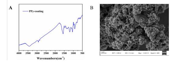
Fig.S2 A. The FTIR spectrum of the PPy-coating. B. SEM image of the top PPy layer.
