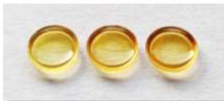
**Figure S1.** Glassy photopolymer of BisOx + 0.5 mol% S-B per reactive group after photo-DSC measurement at 140 °C
