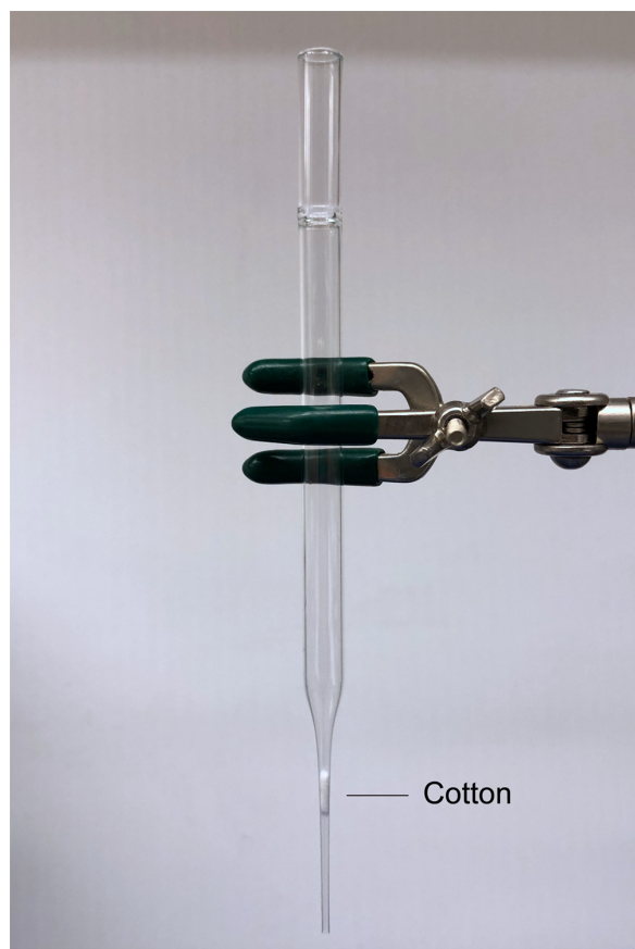
Figure S35. Photograph of cotton-plugged glass Pasteur pipette (Fisher Scientific, Cat# 22-183624) for the filtration of un-encapsulated hydrophobic cargo molecules.
