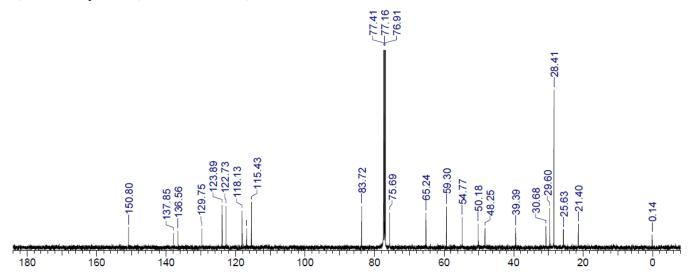
7-17. NMR Spectra of tert-butyl 2-(3-oxoprop-1-en-2-yl)-1,3,4,6,7,12b-hexahydroindolo[2,3-a]quinolizine-12(2H)-carbox-ylate (**C**)
