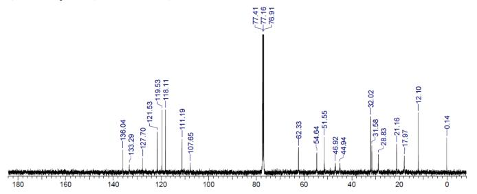
7-22. NMR Spectra of tert-butyl-2-(1-methoxy-1-oxobutan-2-yl)-1,3,4,6,7,12b-hexahydroindolo[2,3-a]quinolizine-12(2H)-carboxylate (**26**)
