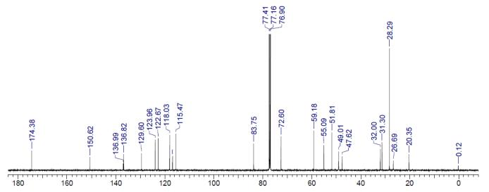
7-16. NMR Spectra of tert-butyl 2-(1-hydroxy-3-methoxypropan-2-yl)-1,3,4,6,7,12b-hexahydroindolo[2,3-a]quinolizine-12(2H)-carboxylate (**22**)
