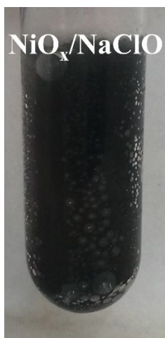
Figure S5. The photo of NiO x and NaClO mixtures. The photo was taken when adding NiO x (80 mg) to 7.5 wt% NaClO aqueous solution (3 g) 1 minute later. The conversion of NaClO was 58% after 30 minutes agitation.
