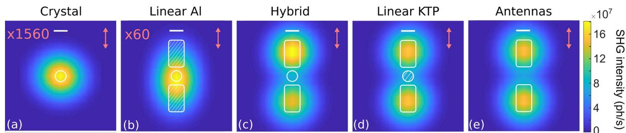
Figure S.2: Simulated excitation cartography of the SHG intensity for different nanostructures. (a) Single KTP crystal of 42 nm radius, 25 nm height and 10 nm minimum radius of curvature. (b), (c), (d) Hybrid Al-KTP structure respectively without the nonlinear contribution of the aluminum, with all contributions included and without KTP contribution. (e) Aluminum antennas without KTP. Color scale multiplying factors are indicated in red if applied.
