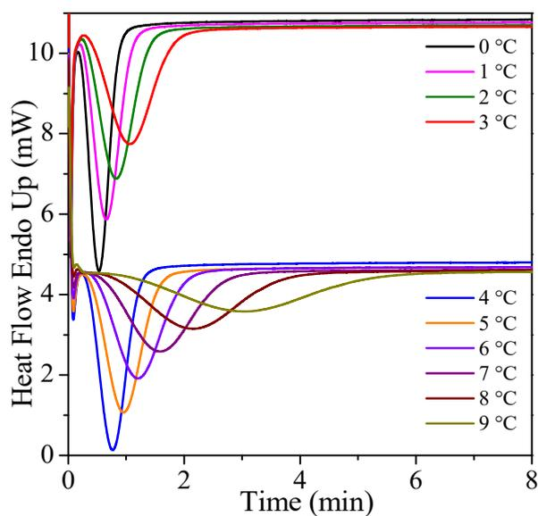
**Figure S7:** Isothermal crystallization curve of AMB-PEG<sub>22</sub>C<sub>20</sub>, following isothermal protocol 1a at different crystallization temperatures. Isothermal protocol 1a: Cooling from the melt at 1 °C·min<sup>-1</sup> to 10 °C, followed by further cooling from 10 °C at 50 °C·min<sup>-1</sup> to the established crystallization temperature.
