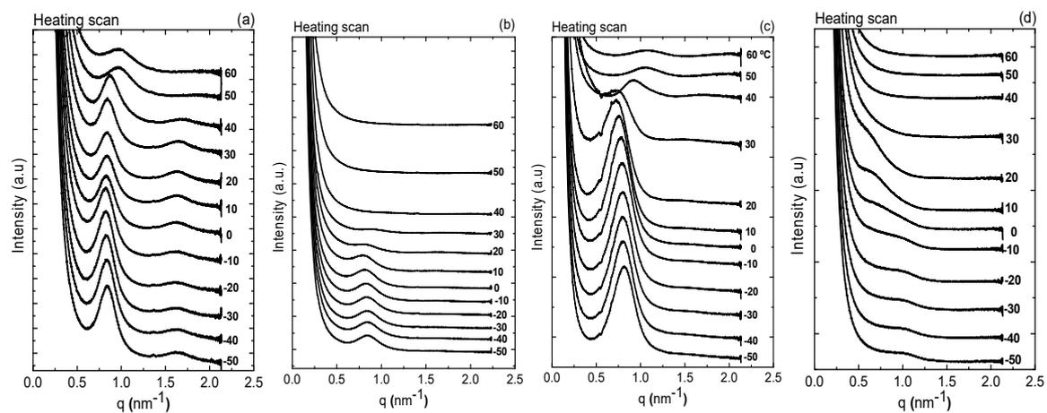
**Figure S5.** Variable-temperature SAXS pattern taken at different temperatures during heating from the crystalline state of (a) AMB-PEG<sub>12</sub>C<sub>20</sub> (b) AMB-PEG<sub>16</sub>C<sub>20</sub>, (c) AMB-PEG<sub>22</sub>C<sub>20</sub> and (d) AMB-PEG<sub>22</sub>C<sub>16</sub>.
