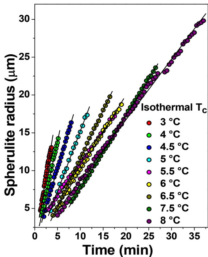
**Figure S6:** Spherulite radius versus isothermal crystallization time of AMB-PEG<sub>22</sub>C<sub>20</sub>, at various isothermal temperatures.
