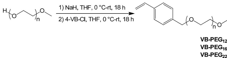
**Scheme S1.** Synthetic route towards 4-vinyl benzyl-[poly (ethylene glycol)] methyl ether (VB-PEG<sub>n</sub>).
