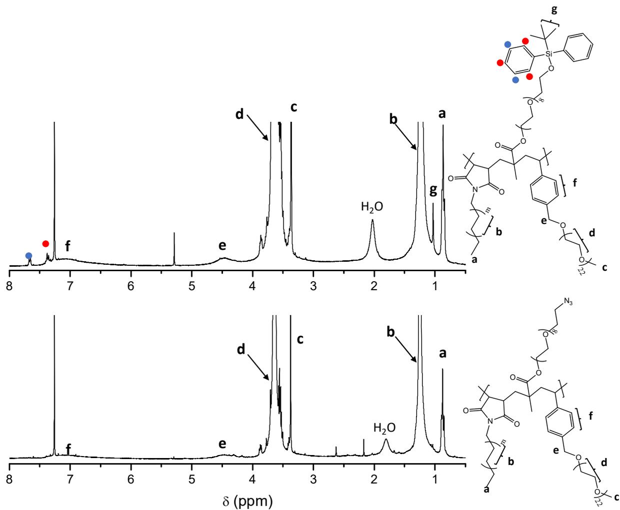
**Figure S2.** A typical  $^1\text{H}$  NMR spectra of the hetero-arm amphiphilic molecular brush before (top) and after (bottom) modification of the methacrylate repeat units (TBDPS to azide). Spectra shows characteristic resonances for all three of the macromonomer repeat units.
