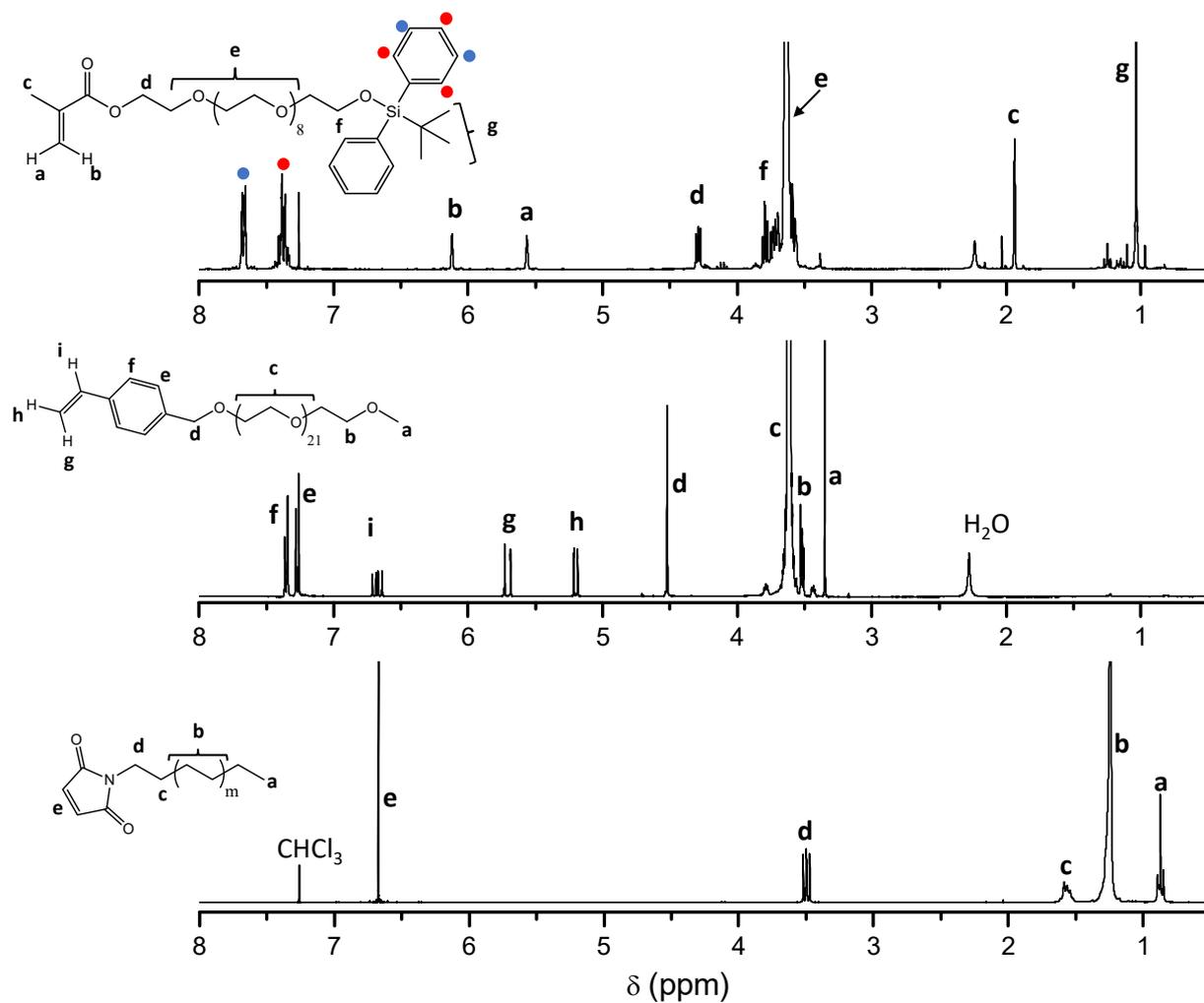
**Figure S1.** <sup>1</sup>H NMR spectra of two of the hydrophilic macromonomers, *tert*-butyl diphenyl silyl poly(ethylene glycol) methacrylate (TBDPS-PEGMA) and 4-vinyl benzyl-(poly(ethylene glycol)) methyl ether (VB-PEG<sub>22</sub>), and hydrophobic macromonomer *N*-alkylmaleimide (MI-C<sub>16</sub>) used for the preparation of the AMBs.
