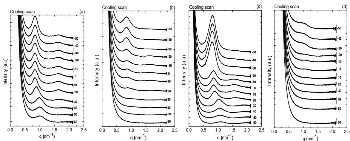
**Figure S4.** Variable-temperature SAXS pattern taken at different temperatures during cooling from the melt of (a) AMB-PEG<sub>12</sub>C<sub>20</sub>, (b) AMB-PEG<sub>16</sub>C<sub>20</sub>, (c) AMB-PEG<sub>22</sub>C<sub>20</sub> and (d) AMB-PEG<sub>22</sub>C<sub>16</sub>.
