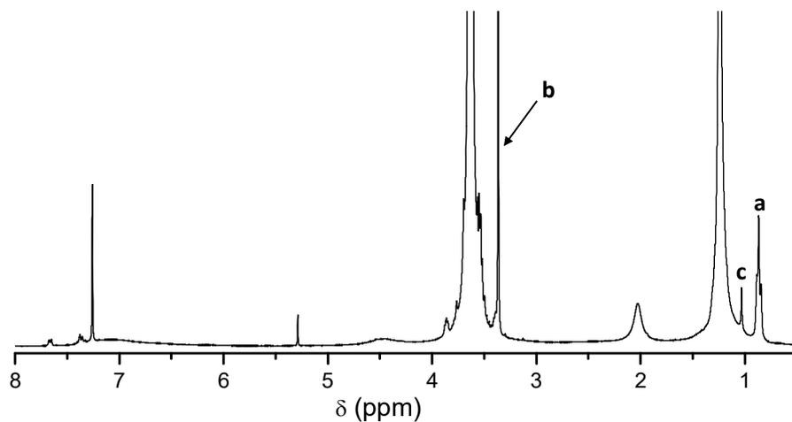
**Figure S3.**  $^1\text{H}$  NMR spectrum of AMB-PEG<sub>22</sub>C<sub>16</sub> showing the peaks integrated for composition analysis of the three repeat units in the AMB. Peak **a** ( $-\text{CH}_3$ , *N*-alkylmaleimide), **b** ( $-\text{CH}_3$ , VB-PEG<sub>*n*</sub>) and **c** ( $-\text{C}(\text{CH}_3)_3$ , TBDPS-PEGMA).
