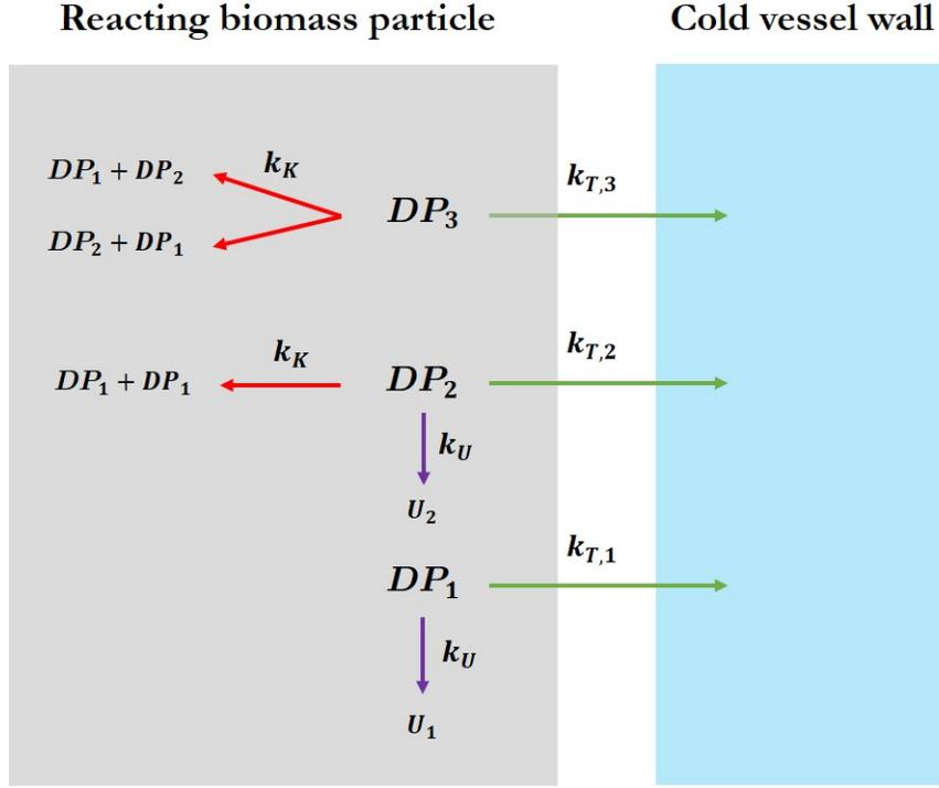
Figure 14: Schematic representation of C<sub>6</sub> sugars (in biomass) pyrolysis
