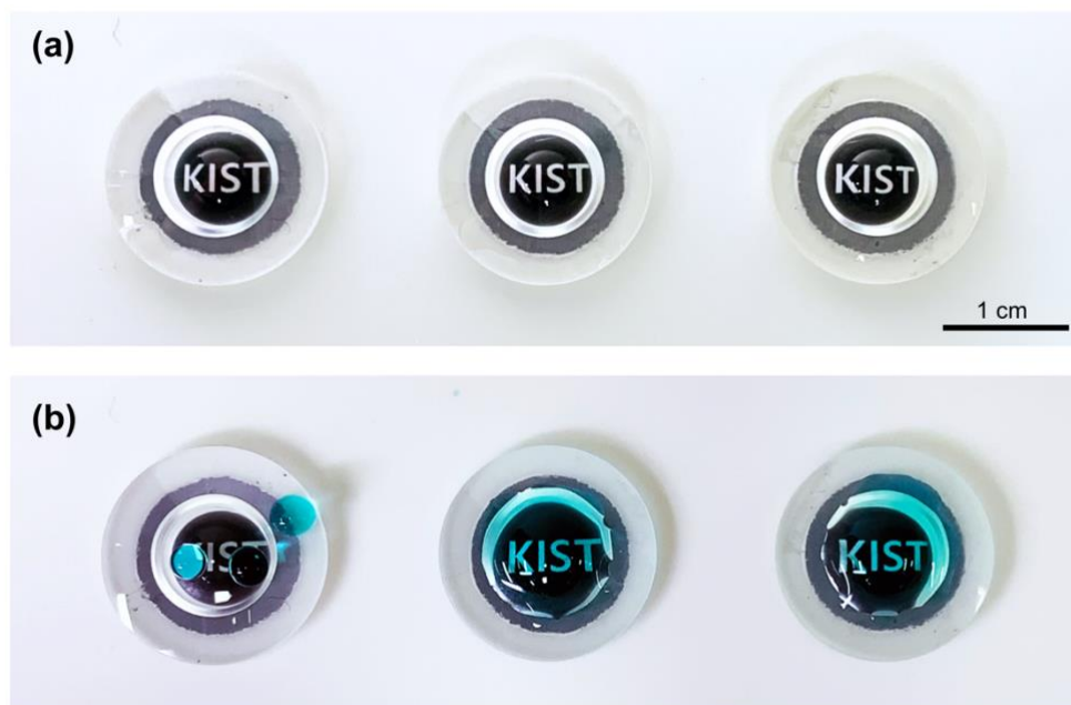
Figure S6. Optical images of water droplets on three lenses (a) without or (b) with water droplets: Bare lens (left) without plasma etching and surfaces prepared with either 250 nm (middle) or 500 nm (right) SiO 2 layer (with CF 4 plasma etching for 15 or 30 min, respectively). Water droplets of approximately 5 \mu L were gently deposited onto the surfaces using a micro-pipet. Nanostructured lenses showed a water layer on the surfaces, whereas the bare lens showed water droplets.
