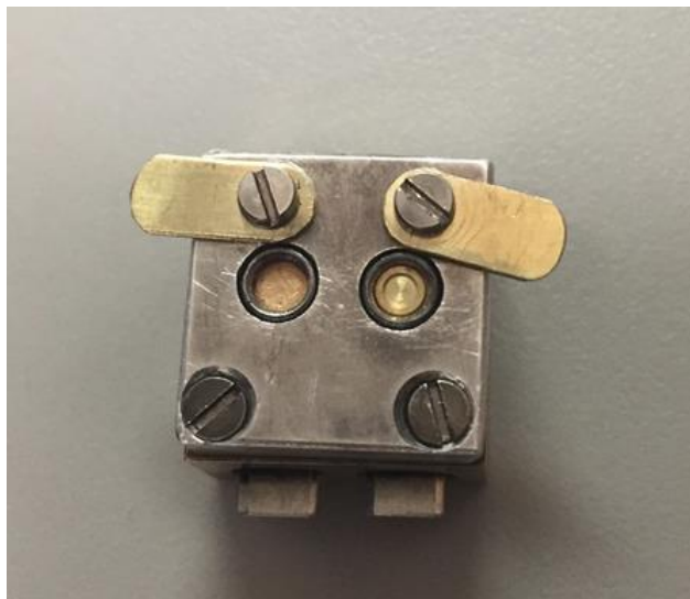
Figure SI 1. Cryo-SEM sample holder. The sample cavity on the right contains one of the Ted Pella brass planchets that is used to freeze and fracture the hydrogel or organogel samples. The sample cavity on the left is empty.
