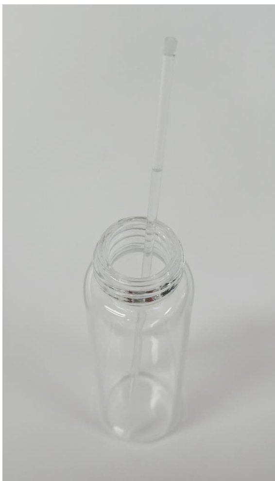
Figure S1. General graphical representation of piASAP: liquid sample sealed with paraffin before the analysis.
