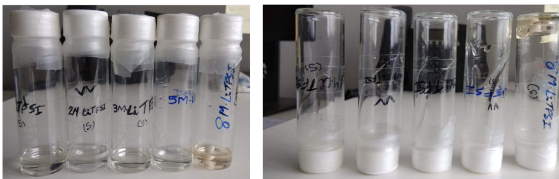
Figure S4 Digital images of the inversion tests of Li-P-X specimens showing the increment in viscosity with respect to an increase of LiTFSI content in PEGDME.
