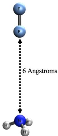
FIG. S1. Geometry of the  $\text{NH}_3\text{-F}_2$  dimer. The N-H bond length and H-N-H bond angle is  $1.02\text{\AA}$  and  $106.2^\circ$ . The  $\text{F}_2$  bond length is  $1.43\text{\AA}$ .
