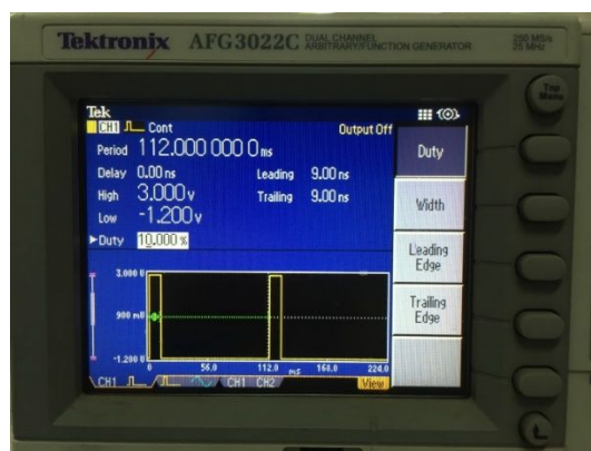
Figure S2. Showing the parameter interface of the signal generator for Cu-PLL electrodeposition.
