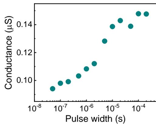
**Figure S5.** The conductance variation after pre-synaptic spikes with different durations.
