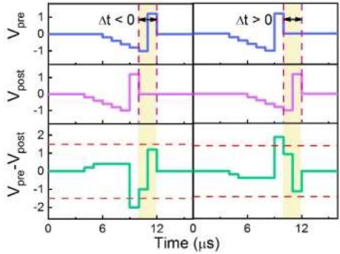
**Figure S6.** Sketch of the antisymmetric STDP learning shape. The voltage of pre- and post-synaptic spike and their sum are represented by  $V_{pre}$ ,  $V_{post}$  and  $V_{pre}-V_{post}$ , respectively. The red horizontal lines are the threshold voltages of  $\pm 1.5$  V.
