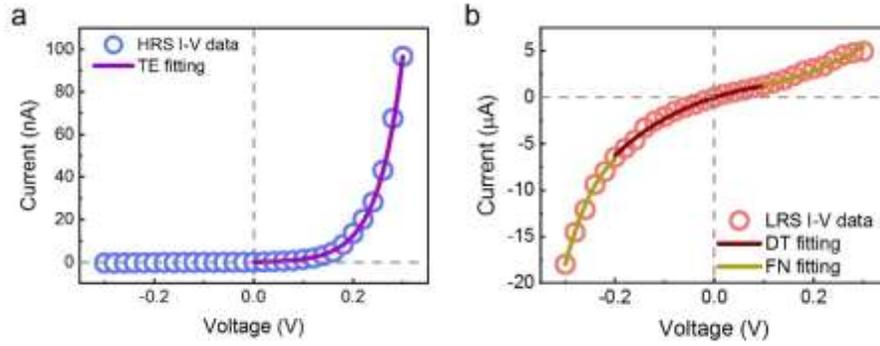
**Figure S1.** Representative  $I$ - $V$  curves at HRS and LRS. a) Measured (open circles) and fitted (line)  $I$ - $V$  curves of HRS. b) Measured (open circles) and fitted (line)  $I$ - $V$  curves of LRS.
