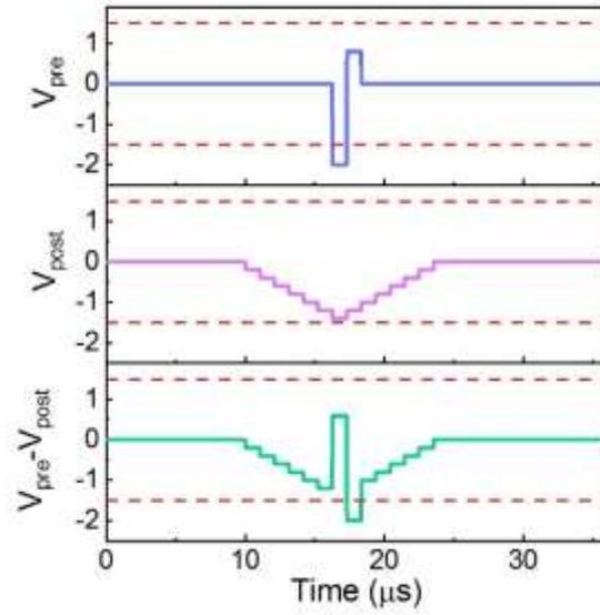
**Figure S7.** Sketch of the symmetric STDP learning shape. The voltage of pre- and post-synaptic spike and their sum are represented by  $V_{pre}$ ,  $V_{post}$  and  $V_{pre}-V_{post}$ , respectively. The red horizontal lines are the threshold voltages ( $\pm 1.5$  V).
