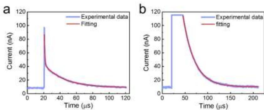
**Figure S2.** Exponential fitting of the decay curves of short term memory (STM). The current-time ( $I-t$ ) curves are triggered by pulses with a duration of 50 ns, amplitudes of 1 V (a) and 1.2 V (b) with a compliance of 115 nA. The relaxation time constant  $\tau_1$  are 23.5  $\mu\text{s}$  for (a) and 25.4  $\mu\text{s}$  for (b), respectively.
