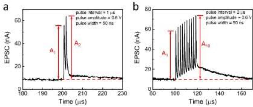
**Figure S3.** The paired-pulse facilitation (PPF) and PTP behavior of the OTJs. (a) The EPSC curve triggered by double spikes.  $A_1$  and  $A_2$  are the peak values of the first and second spikes. (b) The EPSC curve triggered by ten spikes.  $A_{10}$  is the peak value of the tenth spike. The background bias is 0.1 V.
