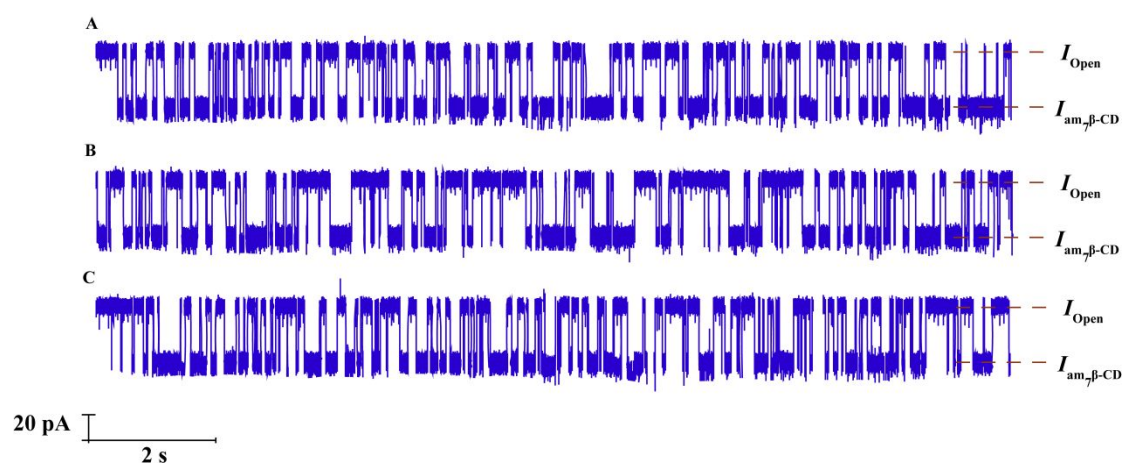
Figure S1 The current signal recordings of (A) am 7 β-CD, (B) am 7 β-CD and trypsin (C) am 7 β-CD and BAEE. These experiments were carried out under 1 M NaCl, 10 mM Tris-HCl and pH 8.0. 40 μM am 7 β-CD was introduced from trans chamber, 0.8 μM trypsin and 66.6 μM BAEE were added from cis chamber respectively and the transmembrane voltage was +140 mV.
