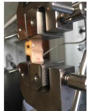
**Figure S4:** Setup for measuring *In vitro* Adhesive property of BioGel and BioPEG.
