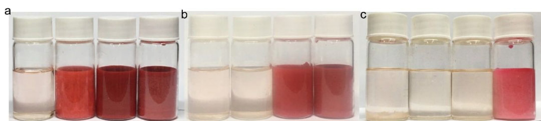
Figure S4. Optical photograph of the TC-PCSs obtained at different temperature, (a) 30 °C, (b) 42 °C (c) 55 °C. The four samples corresponding to different phase change materials, are lauryl alcohol, tetradecanol, hexadecanol, octadecanol respectively.
