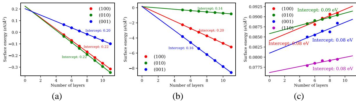
**Figure S1:** Surface energies for low index facets on the three materials considered in this study.
