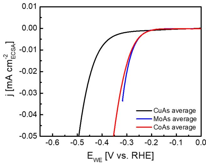
**Figure S3:** HER activity normalized for the electrochemical active surface area (ECSA).
