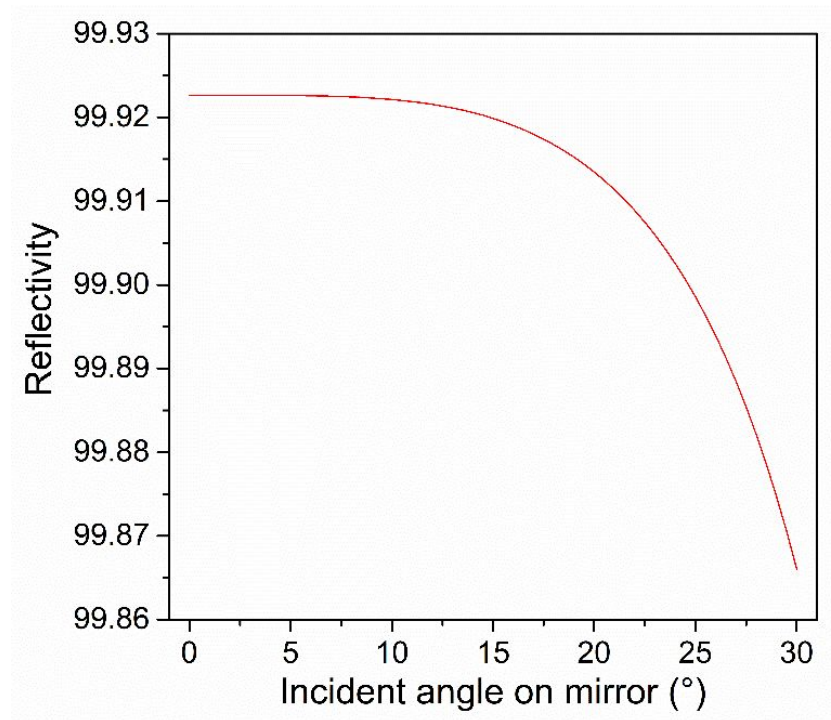
Figure S1. Calculated reflectivity of a 15-layer dielectric mirror as a function of the incident angle using an example model named “Distributed Bragg Reflector” in COMSOL.
